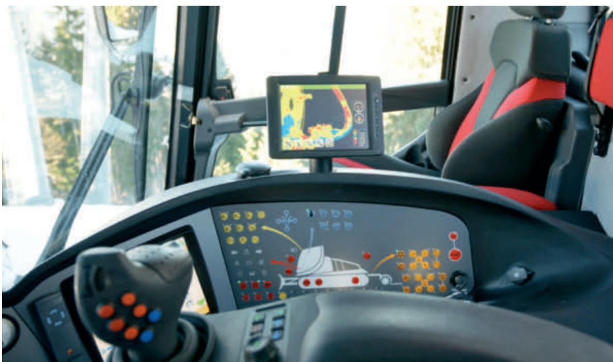
Touchscreen operation for the SNOWsat system in the driver's cab.
