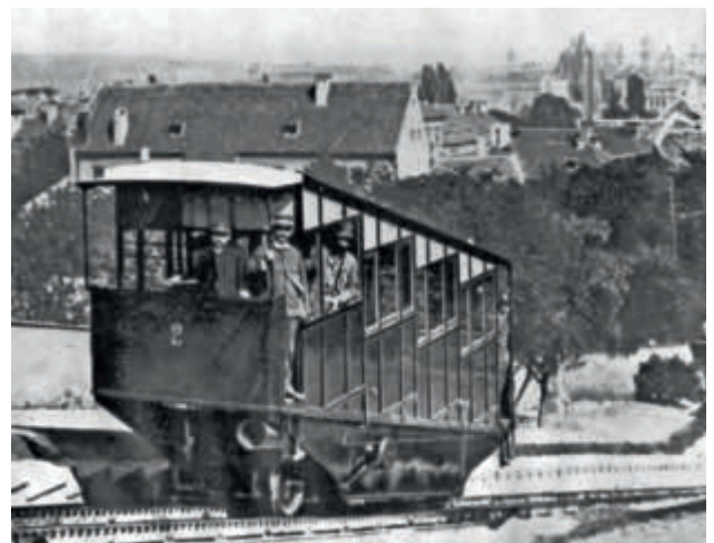
The first Petřín funicular built in 1891. At the front of the car on the right you can see the funnel for filling the tank with water.
