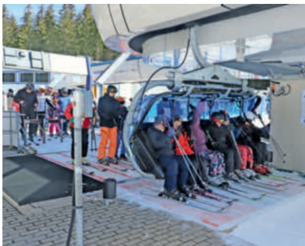
Conveyor loading in the bottom station
