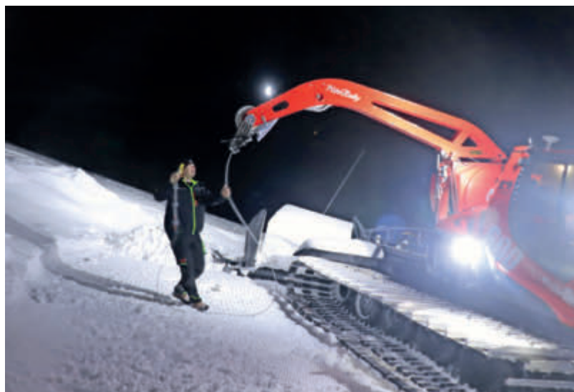
Before moving on to the next section of the slope, the winch cable has to be released from the anchor point.
