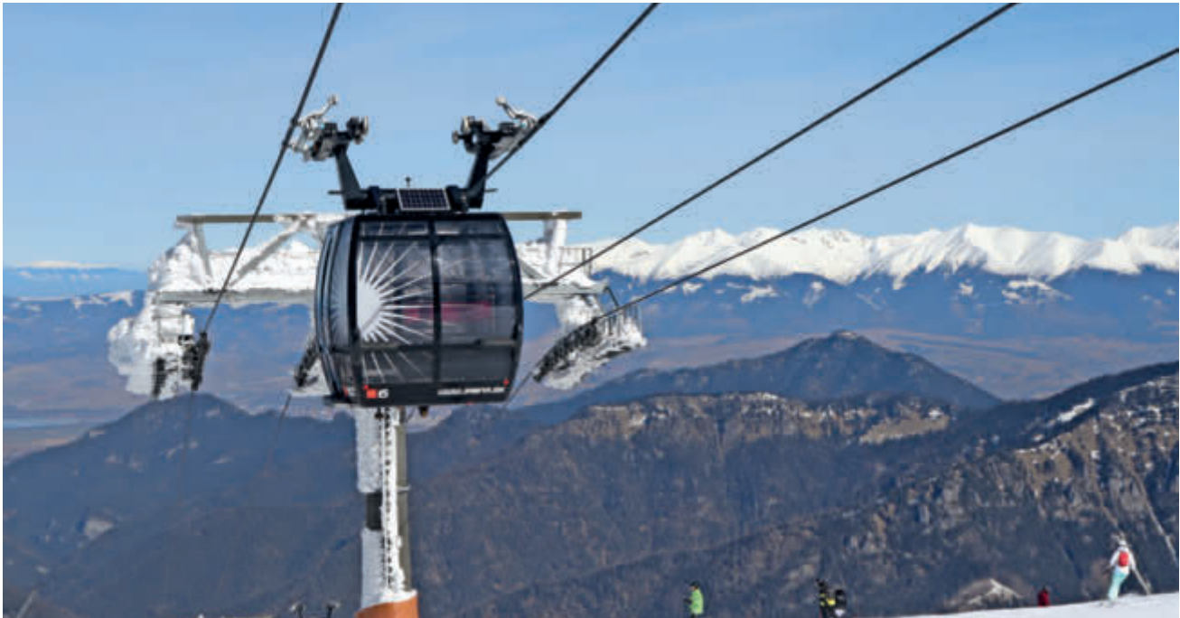
On the north side, the 24-passenger funitel runs from Priehyba to the top of Chopok .
