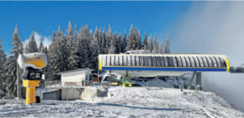
Testing the TR8 snow gun located at the highest point next to the top station of the gondola lift
