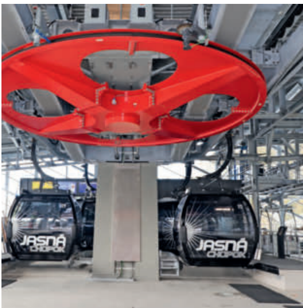
The bottom station at Biela Pút , with the parking rail on the right
