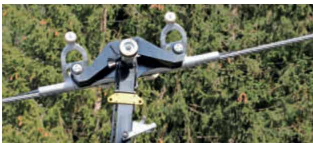
Double grips for the 15-passenger cabins
