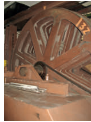
The two brake cable drums in the top station
