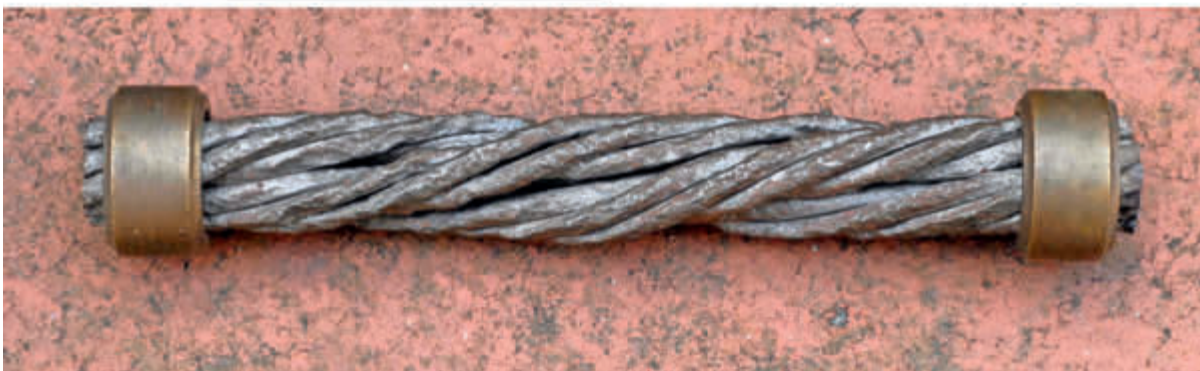
Albert's wire rope: The invention of the wire rope by Julius Albert in 1834 was a prerequisite for the development of the ropeway. The rope had three strands with four iron wires each. In the figure you see the cross-section and top view of an original piece of Albert rope and the cross-sectional drawing.
