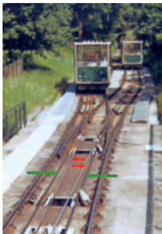
The Abt switch, looking down the line. Green arrows: the two sections of the haul rope; red arrows: the two separate brake cables
