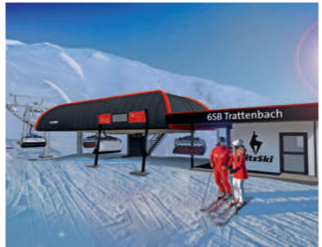
Bottom station of the new Trattenbach 6-seater chairlift
