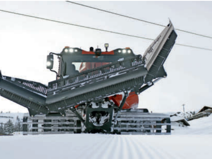
The new ProBlade has integrated hydraulic transport tines. The wings can be tilted backwards for better snow transport.
