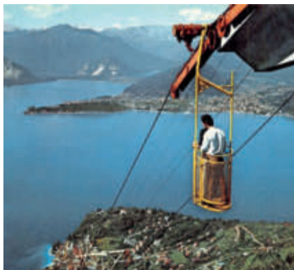
The first ropeway from Laveno Mombello to Poggio Sant'Elsa had yellow open bucket carriers for two passengers.
