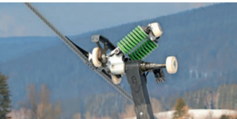
The D-Line D 3000 detachable grips in use in the Kraličák ski area have helical springs in four different colors.
