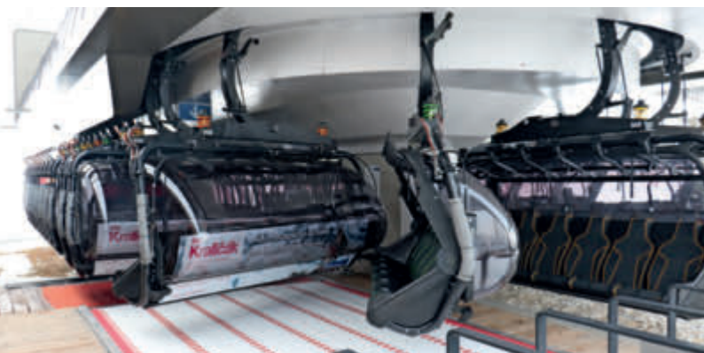
The chairs are parked on the turnaround in both stations.
