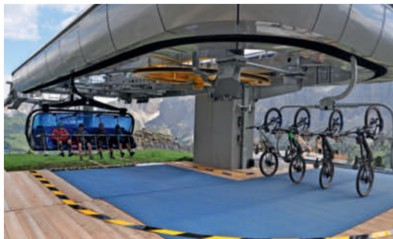
One of the seven bike carriers for a maximum of four bikes in the top station of the Gran Paradiso 8-seater chairlift (Italy). A stop & go procedure is used for safe unloading.
