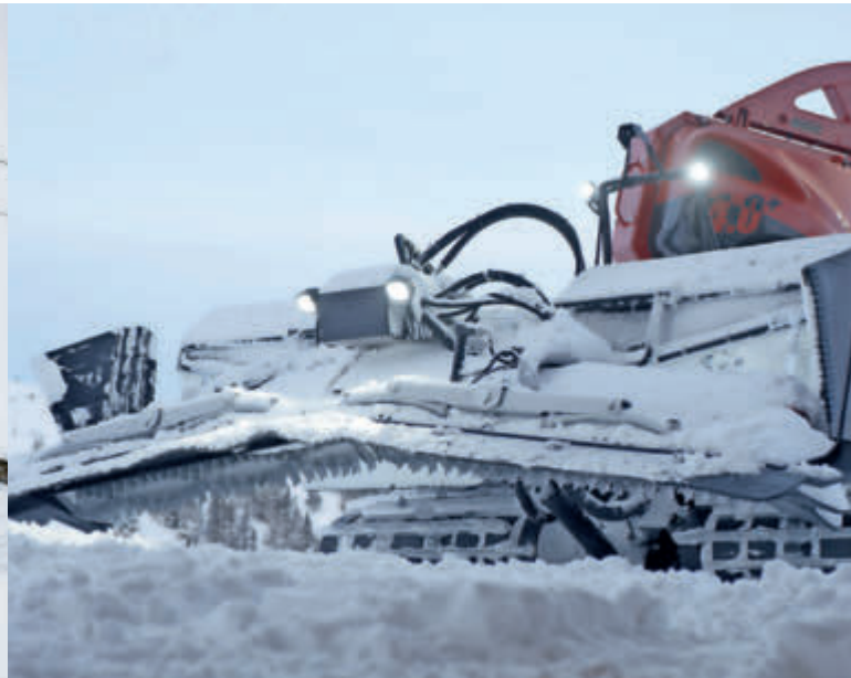
With its enlarged flex angle and V / A position, the ProFlex tiller provides optimum adaptation to the slope.
