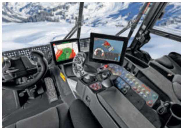
All current PistenBully models are now identical with regard to the controls.
