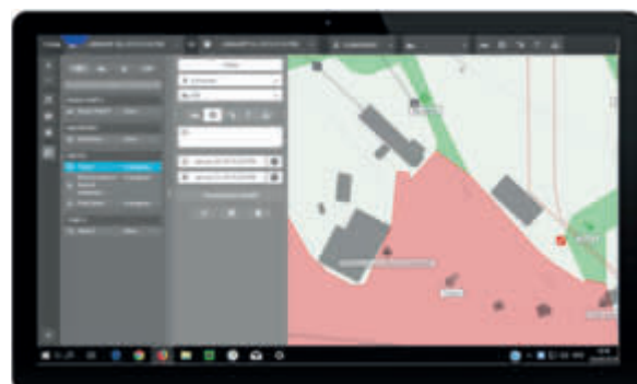
Task assignment on the map – The slope manager assigns jobs in several ways: Tasks for all drivers are shown on the left of the screen (including completion status). The job of adding snow on slope “Access Thuit 4” (add snow) is displayed to the slope manager as completed (Done – area marked in green on the map). Individual tasks for drivers can be added in this area, including details such as comments and the date.
