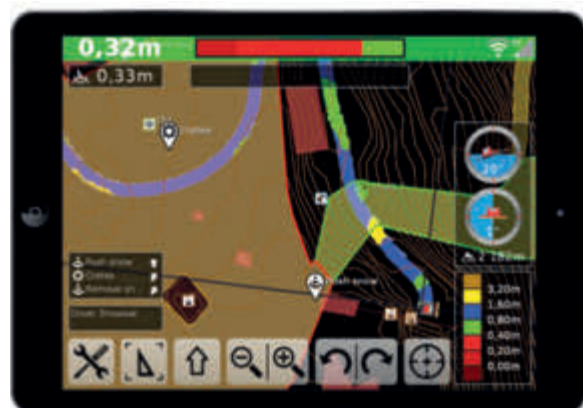
Display in the vehicle – The driver sees the tasks assigned to him directly on the vehicle display. He can edit them on the slope and mark them as completed.
