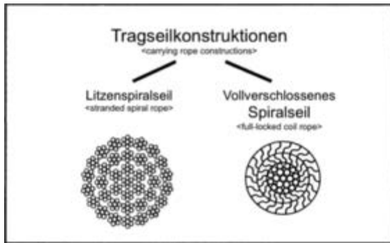
Fig. 1: Cross-sections of track rope constructions, with a multi-layer stranded rope of equal round strands (Herkules rope) on the left and a full-locked coil rope on the right
