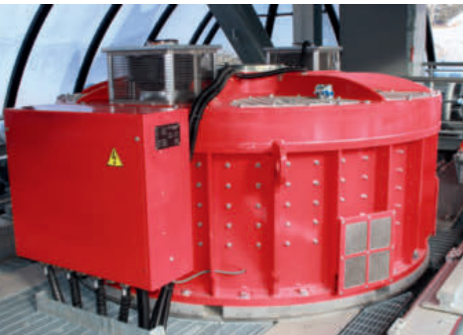
The bottom station houses the direct drive with a continuous output of 347 kW.
