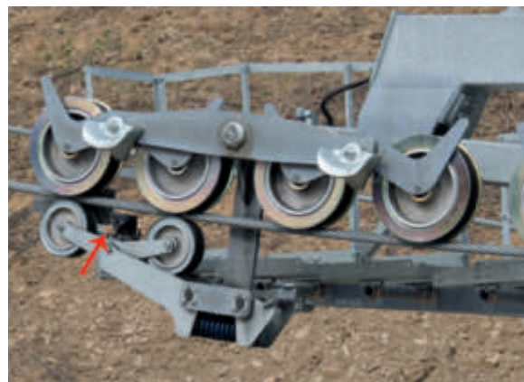
On the depression sheaves, the RPD sensor (red arrow) is located on two auxiliary rollers beneath the line of the haul rope. The photo shows the depression sheave at the exit from the bottom station of the Remiaszów 6-seater chairlift.
