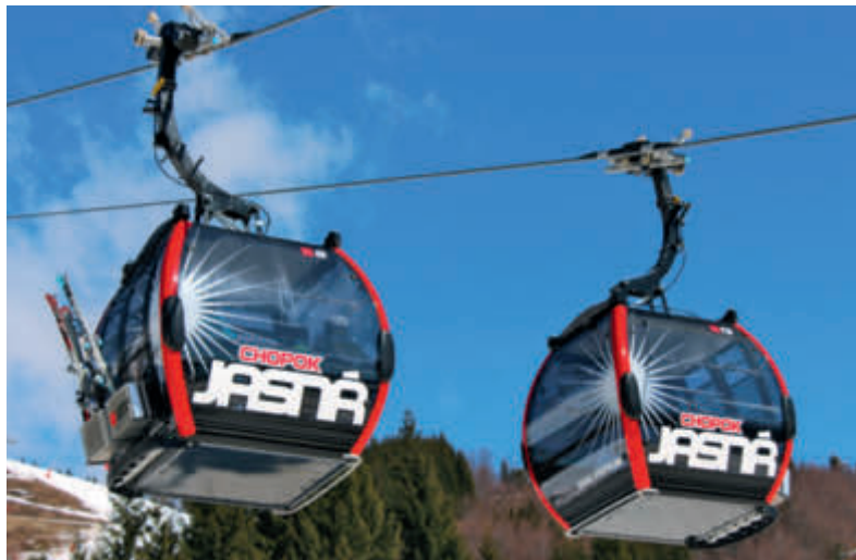
The cabins carry ten passengers seated in comfort and five standing. In view of their 15-passenger capacity, the cabins are fitted with DT 215 double grips.
