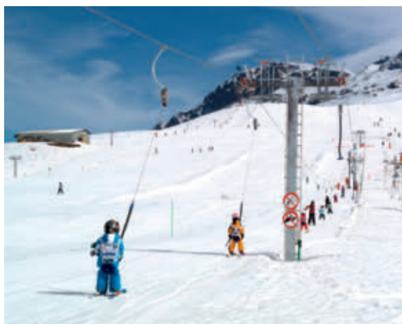
This surface lift is perfect for use in beginners' areas but can also be used on longer and steeper slopes thanks to its 8-30 kW Nord motor.
