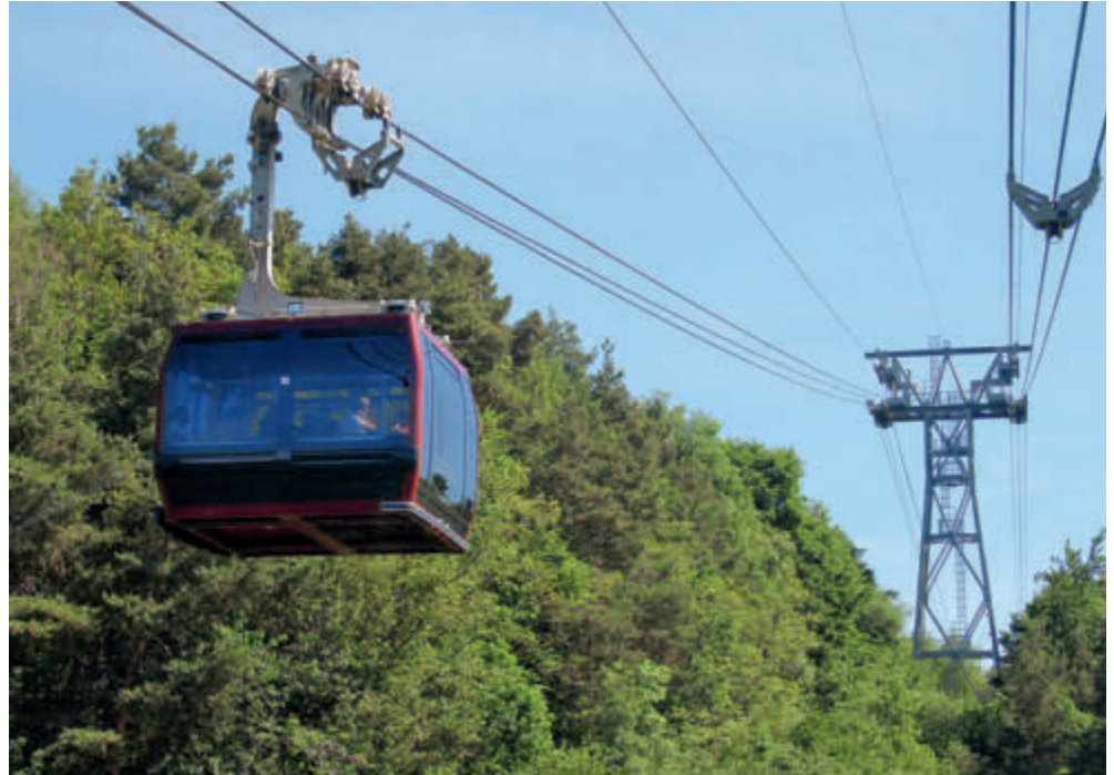
The Ritten Cable Car links Bozen with the Ritten and is popular with both visitors and commuters. It was the first tricable gondola ropeway built by Leitner Ropeways.
