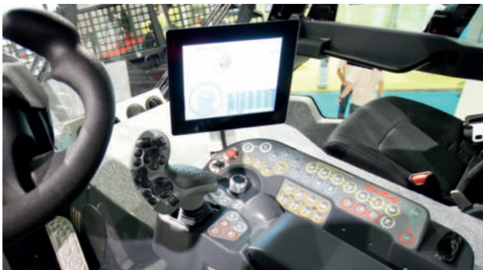
The new cab of the PistenBully 100 with the ergonomic layout of the controls
