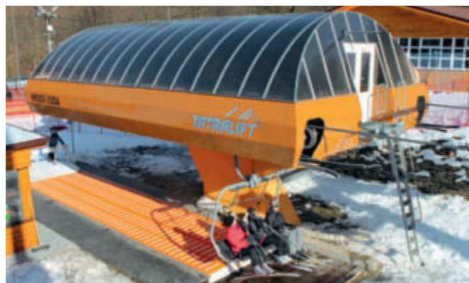
Tatalift is an old-established ropeway manufacturer: Here the Hrubá Voda quad chairlift in the Czech Republic, which was built in 2013.
