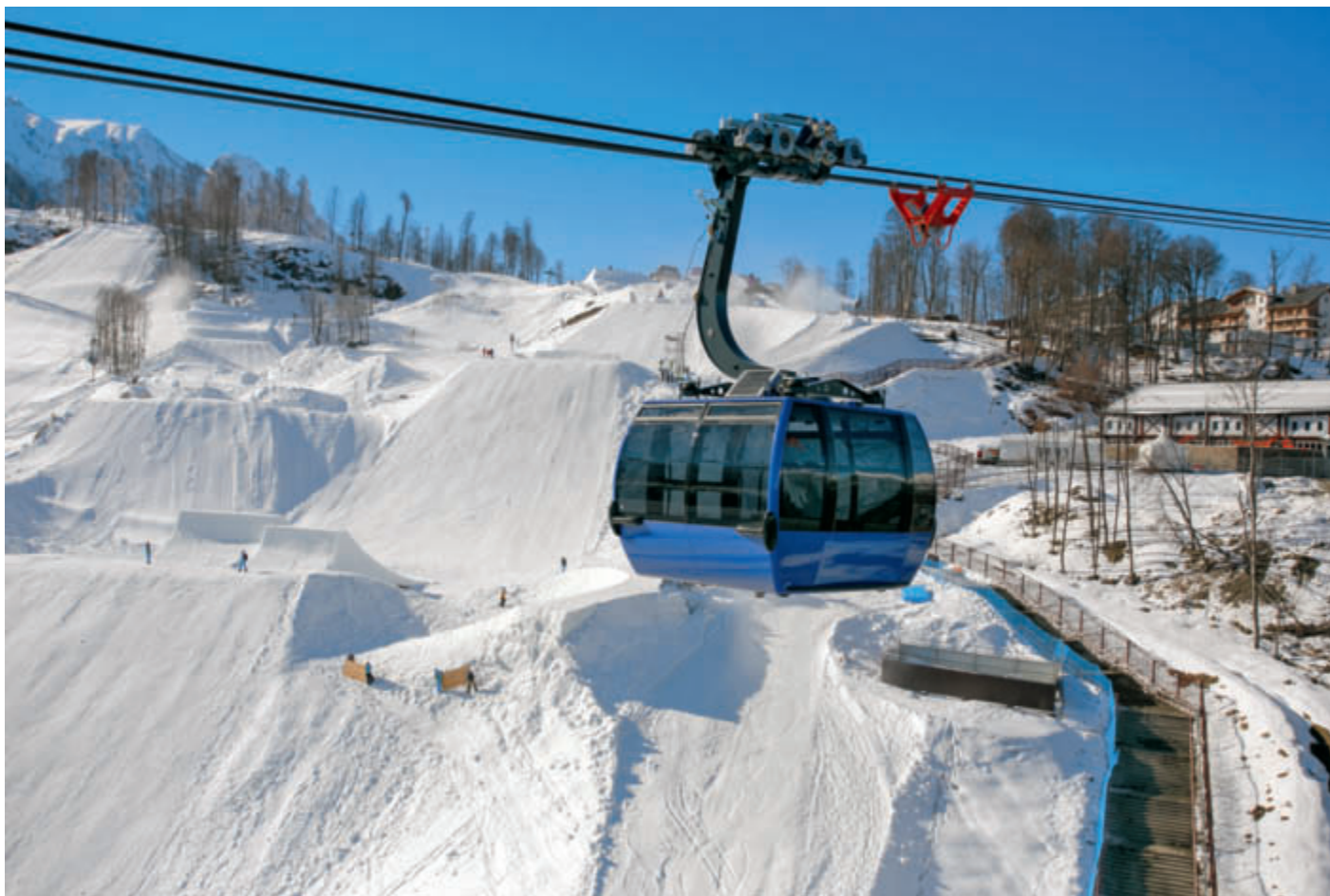
An Olympic champion in its own right: the Rosa Khutor Olympic Village tricable aerial tram with 54 thirty-passenger cabins and 25 car carriers
