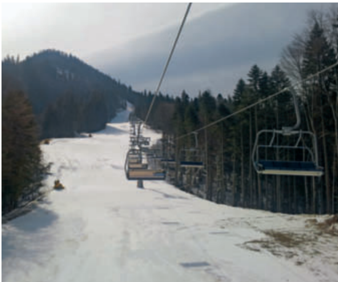
The fixed grip quad-chairlift located in the lower part of the ski area, Lupului Chairlift
