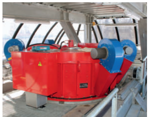
The Pasieka Express six-seater chairlift in Białka Tatrzańska operates with a 300 kW direct drive.
